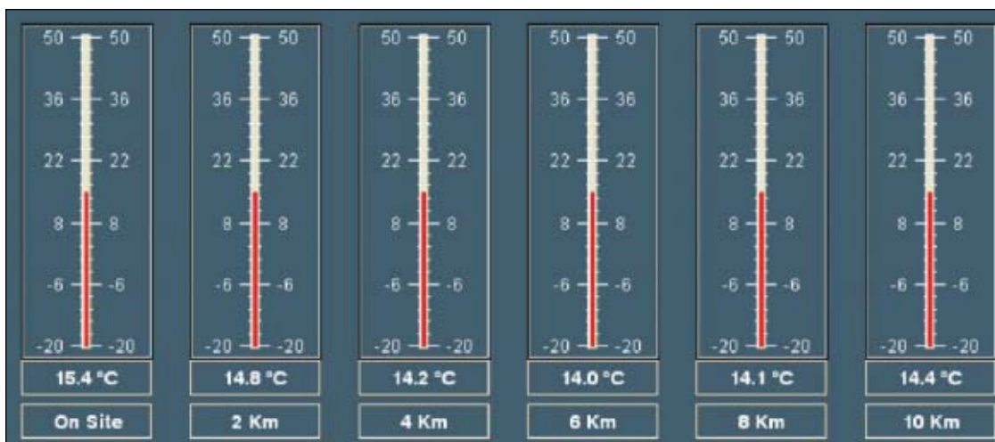
Computer software elaborates and visually displays signals received from the six radio thermocouples positioned along the test pipeline (Fig. 4).
